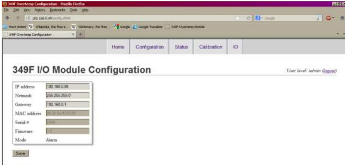
The Configuration page allows the IP address, Netmask, and Gateway setting of the OTM12s network interface to be configured. **Take special note that when changing the IP address you must not lose track of what it has been changed to. If the IP address is lost it may be reset to the factory default 10.10.10.20 by holding the 'Clear' button for >10 seconds.**
